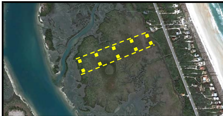
Figure A3-1. Two transects spanning from the marsh edge to the upland edge (approx. 570 m) established at a sample site. Five whole plots (10 x 10 m) are distributed evenly along each transect.
